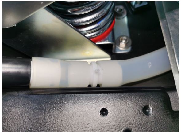
Fig.16 Assemble the T-Connector at another side of Air tube.
