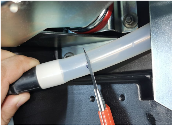
Fig.13 Cut the air tube at cutting line.
